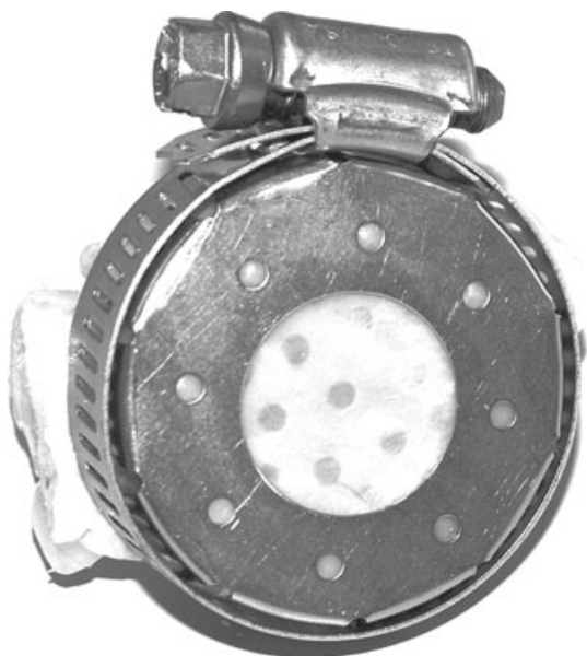
FIG. 1—Mounted and uncovered pigskin placed in the refrigerator.
