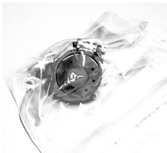
FIG. 2—A vacuum-packed mounted pigskin placed in the refrigerator.
